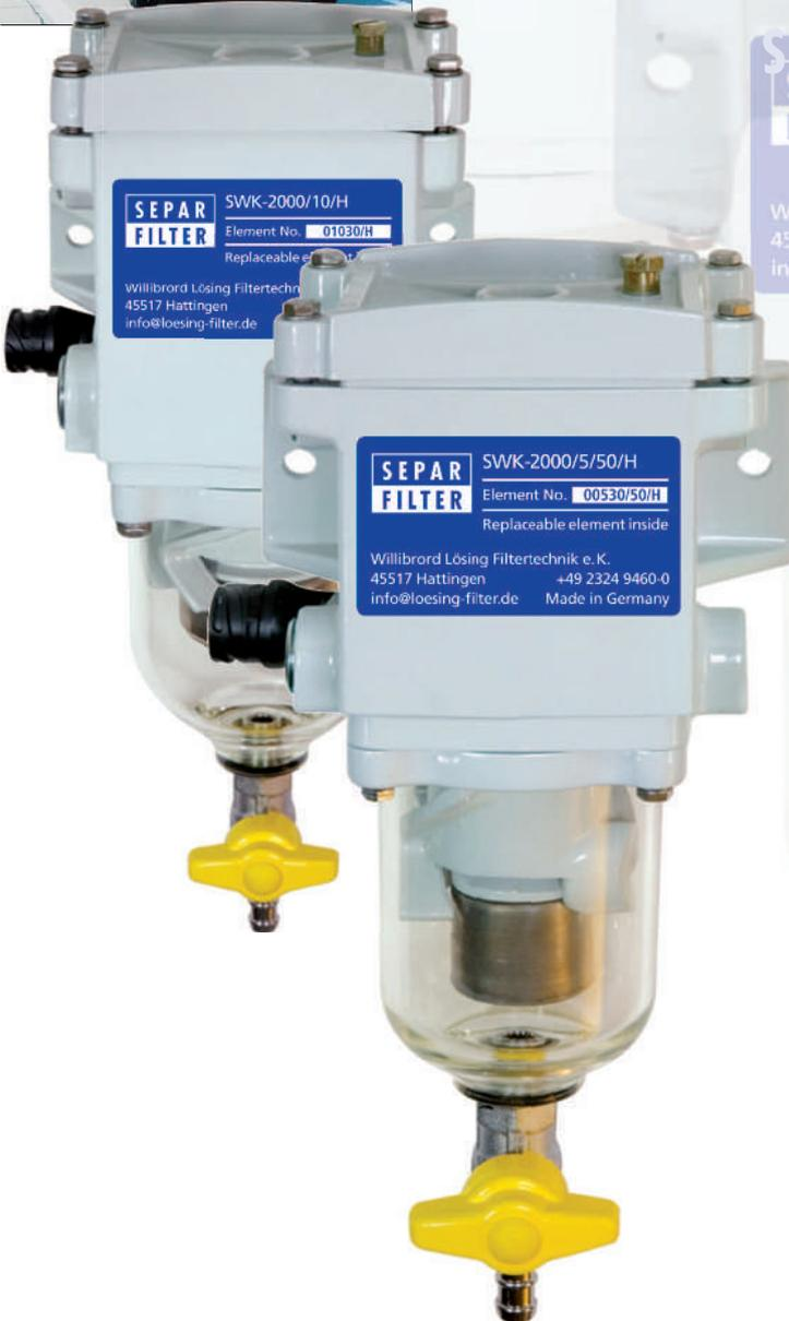
The SEPAR 2000 filter equipped with an electric fuel heating system improves the start up of diesel engines in cold weather conditions at or below 0 °C **and** separates the water and particulate which is contained in the fuel – as described in the attached folder.
